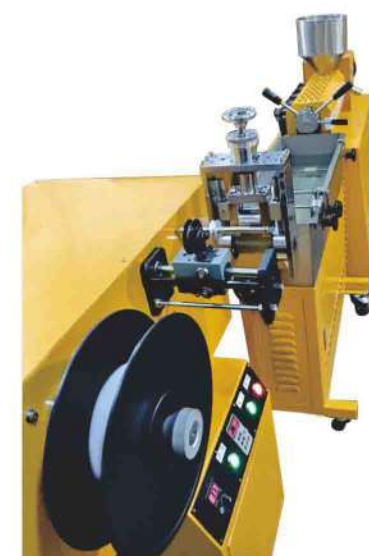
3D耗材收卷辅机 3D consumables reeling auxiliary machine
